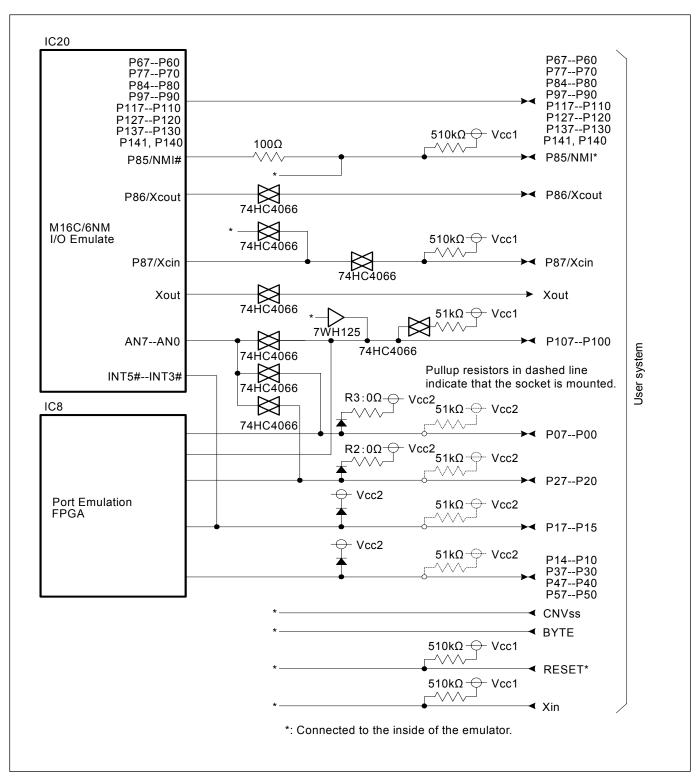
Figure 4.7 Connection diagram
